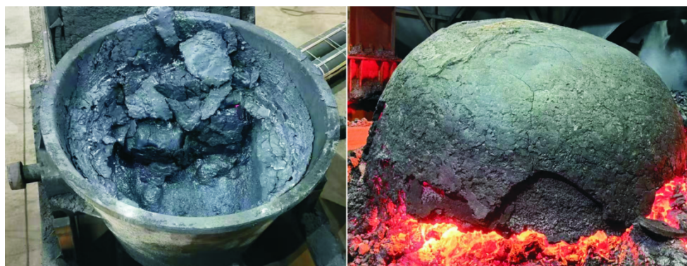
图 1 渣罐底部形成的“铁钝” Fig. 1 Iron thallium formed at the bottom of the slag tank
